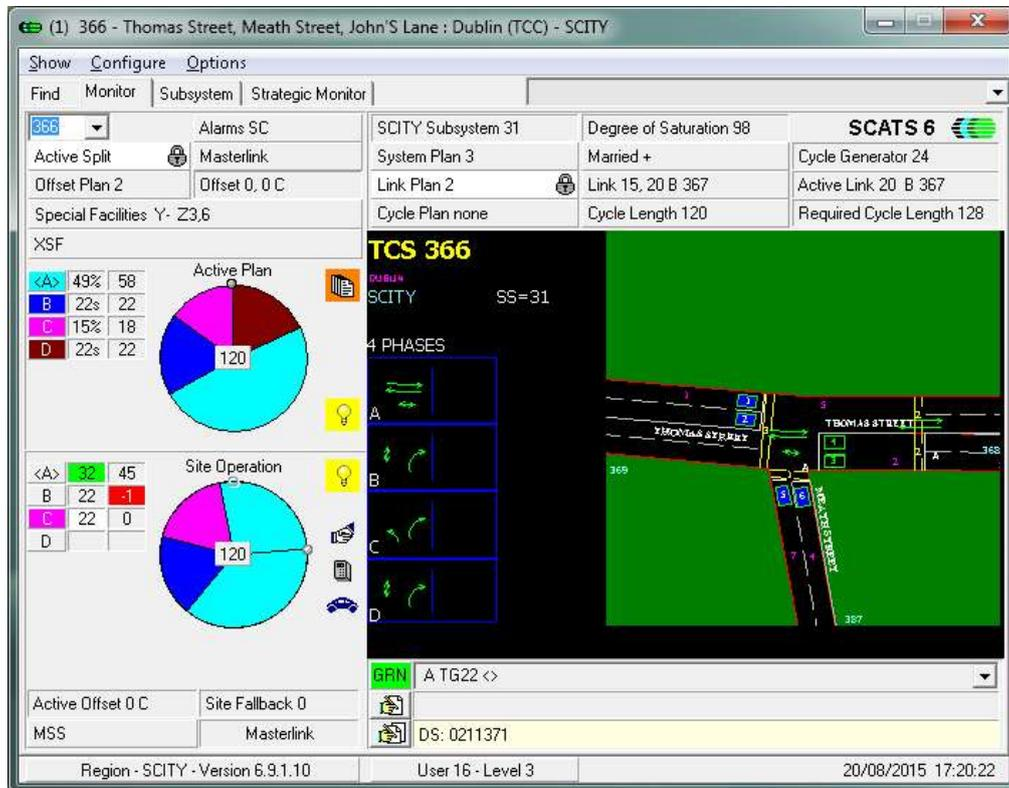
Figure 3: SCATS graphic of Thomas St/Meath St junction with four phases
